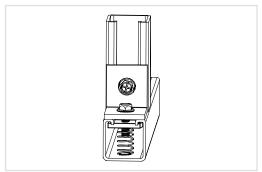
To tighten bolt with wrench for complete assembly.
