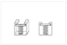
A 90° twist to allow serrated edge of the channel nut to grip in-turned lips of the channel.
