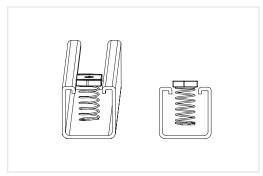
Insert channel nut anywhere along the continuous channel slots. Spring holds back nut in place.
