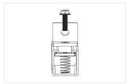
Place appropriate fitting over channel nut and insert bolt 3. for connection.
